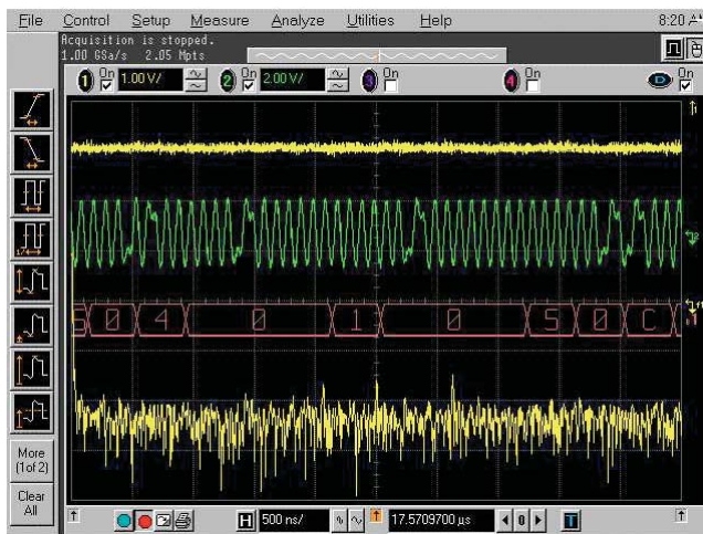
Figure 13. Using the MSO's digital channels can help you gain further insight into the possibility of coupling. Moving the horizontal delay back and forth showed that the noise spikes on the FFT changed in magnitude based on which data was present on the LAN signal according to the hex readouts of the digital bus.
