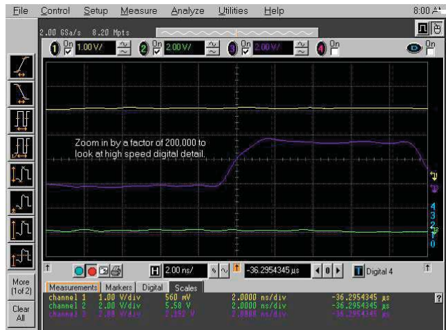
Figure 9. This screen shows the same acquisition shown in figure 8 zoomed in by 200,000 times! MegaZoom Deep memory sustains a high sample rate so you can zoom in to see the details and make accurate measurements.
